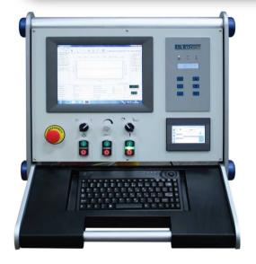
With this new version the recording and controls are made with an on-board Industrial Panel PC with a large 12.1 inch LCD screen . The control panel is also equipped with an in house made electronic microchip circuit which registers and controls signals from pressure transducers and thermocouples.
