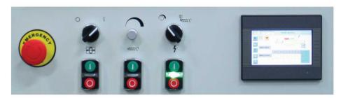
The lower part of the control panel has start/stop buttons for gear pump and extruder as well as main on/off and emergency switches. It also contains a speed control button for the screw RPM and
