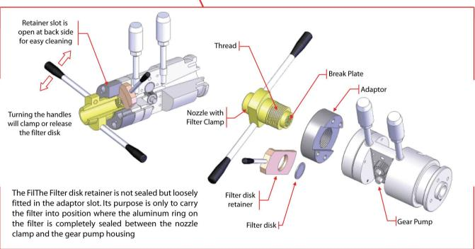
With this system we will eliminate the possibility that the filter is wrongly inserted into the filter retainer. The retainer shown in the drawing is used only to push in the filter disk and it is loosely fitted into the adaptor slot. The retainer and the slot in the housing is designed so that it is not possible to insert the filter disk unless it is properly positioned in the retainer hole.
