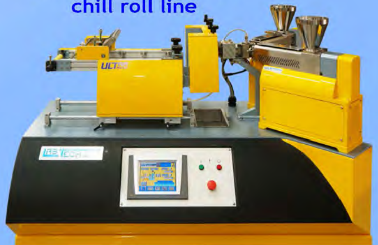
The Ultra Micro Co-Ex chill roll line
