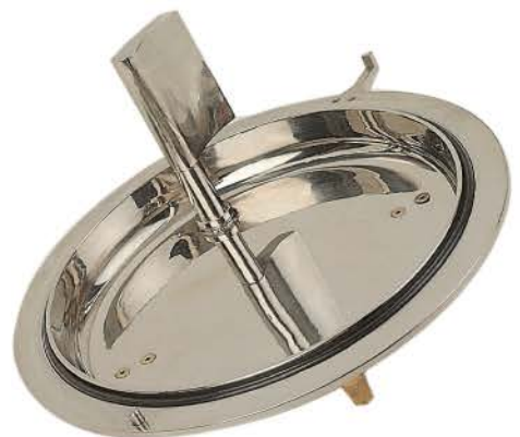
The lid to the mixing bowl is equipped with an adjustable deflector blade. The lid also has an air filter to enable air pressure to be released during mixing.
