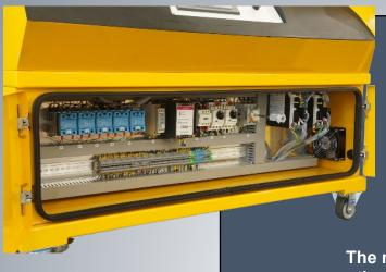
The sub cabinet also contains all the electrical and electronic components comprising of AC Servo & DC motor controls, relays and controls for water pump, electric water heating, PLC unit for touch screen and various safety controls.
