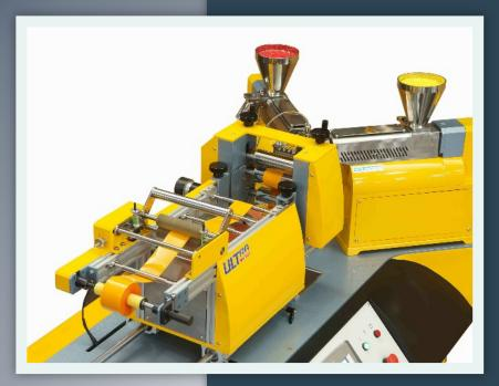
The line features a section type of feed block which divided the in flow from the two extruders into layers A+B+A. This feed block type ensures a very even layer thickness. The layer thickness is regulated by the speed from the extruders which are driven by infinitely variable speed servo motors with a very constant RPM
