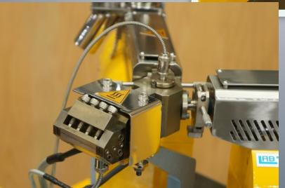
The flat die is of coat hanger type and has a set of adjustment screws for the lip gap. With this the gap can be set from 0.1 to 0.3 mm
