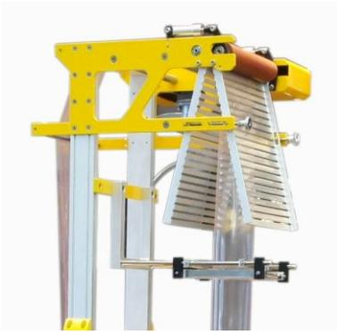
The film tower has a total width of 150 mm and can accommodate a film of a lay flat width up to 100 mm. The rubber nip-rolls are spring loaded and driven with a variable speed DC motor. The A-frame is made with adjustable collapsing angle and there are two film bubble stabilizing frames with adjustments to accommodate different film bubble diameters
