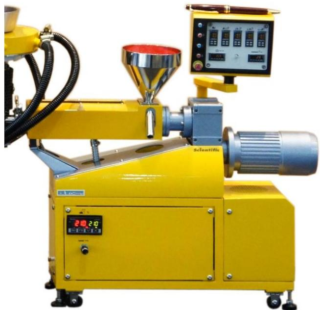
The hopper has a turret valve, same as with our larger extruders and it has a discharge pipe on the side to empty out the hopper.
