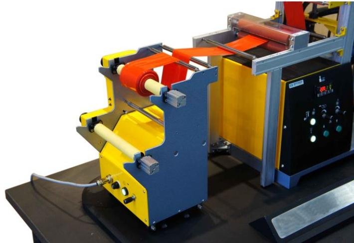
The wind up unit has two spring loaded bobbin film cores which are both driven with a variable speed geared DC motor.
