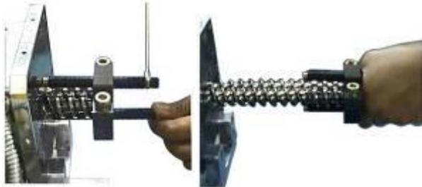
However it is not necessary to open the clam shell to clean the screws. Instead, for fast and easy cleaning, the screws can simply be pulled out from the front with the help of a quick clamp tool supplied with the machine.
