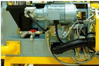
The 20 mm twin is now available in high output, high torque version which has a drive power of 11 kW and a max screw RPM of 1200. This version is equipped with our high torque gear design which has an additional supporting gear shaft. It is also equipped with forced lubrication by an external oil gear pump coupled to a large plate-type oil cooler.
