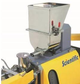
The extruders are supplied complete with a stainless steel volumetric hopper feeder with a single feed screw and with a stirring arm (agitator) above the feeding
