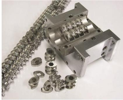
The screws are built on hexagonal elements is supplied in screw made from high-grade tool steel which is through-hardened but made with a slightly softer hardness than the barrel linings to ensure optimum lifetime for both elements and barrel inserts.
