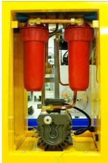
The vacuum venting system is supplied with one stainless steel vent port housing which is equipped with a sight glass on the open swing lid and a vacuum regulator valve with gauge. The vent housing is made with a resin trap to prevent that any resin leaking in the vent will plug the pipes to the vacuum pump. The housing is connected to twin large vacuum filters and a vane type vacuum pump mounted in the sub cabinet.
