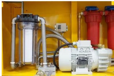
The 32 L/D extruder is, as standard, supplied with a vacuum zone on one of the barrel modules and the 40 and longer L/D versions also have an additional atmospheric vent opening which can be converted to vacuum. The vacuum vent zone has a stainless steel vent port housing which is equipped with a sight glass and vacuum regulator with gauge. The housing is connected to large twin vacuum filters and a vane type vacuum pump mounted in the sub cabinet.
