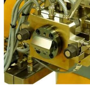
The strand die swings aside simply by loosening the two bolts to facilitate easy cleaning. For connection to other downstream equipment, such as flat die for a chill roll attachment, the extruder can optionally be supplied with a suitable die adaptor.
