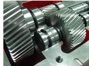
Scientific 26 mm co-rotating twin-screw extruder is made with a complete modular build-up of the clamshell barrel, where each barrel section has a length of 4 D or 104 mm. Many L/D sizes are available from 32 to 60+. The standard twin has a drive power of 15 KW, and a max screw RPM of 800, as well as a re-designed high torque gearbox comprising of additional shaft supporting gears and a direct driven gear pump for closed loop, forced oil cooling system.
