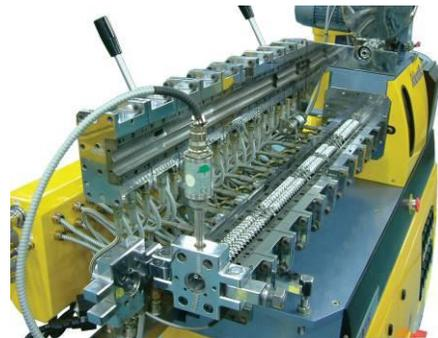
Each barrel zone is equipped with both water cooling and electric cartridge heating. This allows for complete process control at each zone of the barrel and the water cooling coupled with the high wattage heating enables fast temperature changes of each zone when changing processing conditions from one compound to another. The water cooling is done from fine channels inside each barrel module and regulated with individual solenoid valves from its designated temperature controller.
