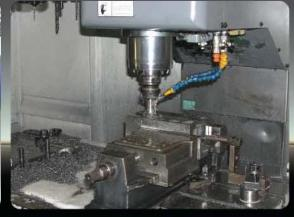
We have many CNC milling and lathe machines on which we produce a large range of parts for our machines, such as twin screw elements, barrel modules and inserts, gear boxes and single layer as well as co-ex film blowing and sheet dies. All machining is carried out in clean rooms with air-conditioning to provide a pleasant working environment for the operators as well as to ensure a very clean environment, free of dust and contamination.
